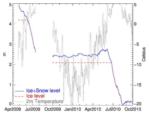
Fig 2: Left: AWS 1 with SR50 on Zhadang Glacier in May 2010; middle: air and ice temperatures measured at AWS 1 over one year; right: daily means of snow accumulation and ablation at AWS 1 in 2009 and 2010 from an ultra-sonic depth sensor (Campbell SR50)
