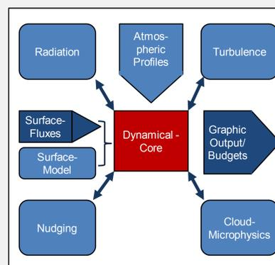
Figure 4: Modular structure of the ATHAM model, simulating the transport of active tracers and convective events (Herzog et al., 98 ; Oberhuber et al., 2008)
