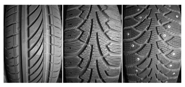
Figure 2. Tested tyre types. From left to right: summer, friction (non-studded winter) and studded tyres.
