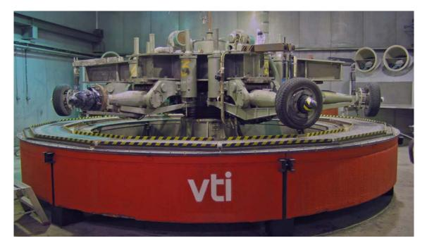
Figure 1. The VTI circular road simulator.
