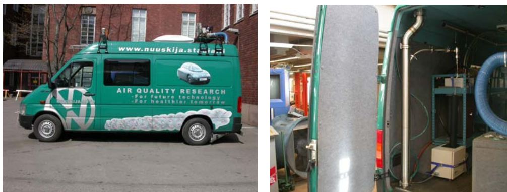
Figure 1. a) The conical inlet behind the left tire of Sniffer. b) The sampling system.
