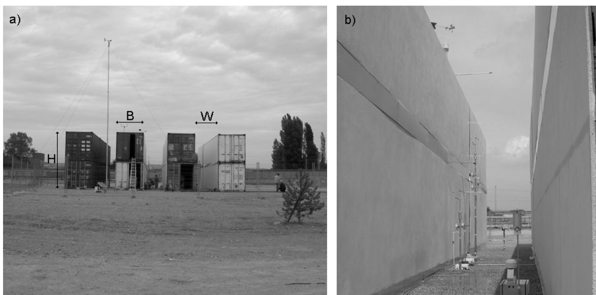
Figure 1. Guerville experimental site: a) site overview, b) instrumentation in the investigated street.
