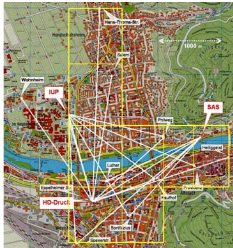
Figure 3: Measurement geometry in Heidelberg with three Multibeam telescopes located at the top of the buildings “IUP”, “SAS” and “HD-Druck”. The light beams (white lines) are redirected to 18 retro reflector arrays. The yellow lines indicate the boxes used for the tomographic 2D reconstruction of the trace gases displayed in Figure 5.
