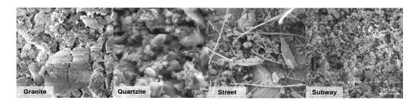
Figure 3. SEM photos of  $PM_{10}$  from combinations 1 (Granite, upper left), 2 (Quartzite, upper right), urban street (lower left) and subway (lower right). The magnification was 2000 times.
