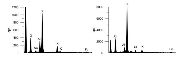
Figur 4. EDS spectra of wear particles from the granite pavement (left) and the quartzite pavement (right).
