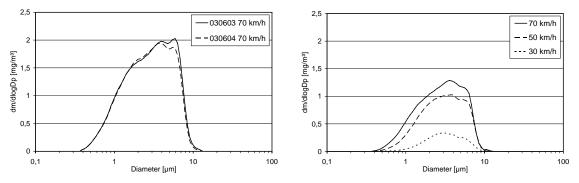
Figur 2. Mass size distribution of pavement wear particles caused by studded tyres. At left from the granite pavement and at right from the quartile pavement.
