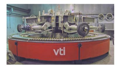
Figure 1. The VTI circular road simulator.
