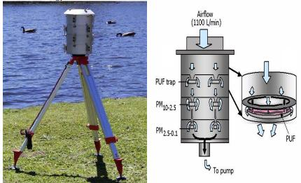
Figure 1. The three stage high volume cascade impactor, collecting  $PM_{10-2.5}$  and  $PM_{2.5}$  onto polyurethane foam substrate.
