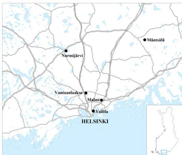
Figure 1. The map of Testbed measurements. All the measurement sites have a ceilometer; the RASS is situated in Malmi and the radiosoundings are performed in Vantaanlaakso.
