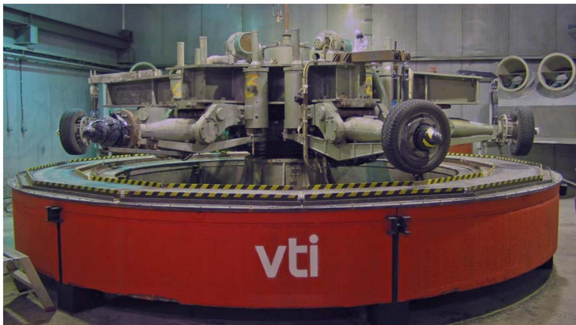
Figure 1. The VTI circular road simulator.
