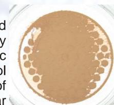
Glass fibre filter coated with HULIS. In fact, the colour of the filter samples resembles to humic substances.
