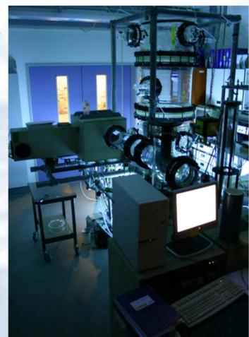
700-L smog chamber with FTIR long-path White cell
