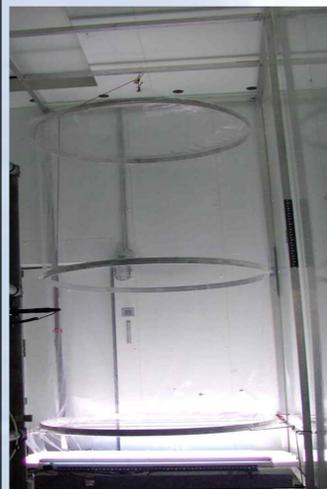
If made of glass, the walls of smog chambers are known to release Cl<sub>2</sub> from ozone and HCl by heterogeneous photochemistry. This artefact is avoided in our chamber, made of Teflon film (3500I, FEP 200A, Dupont), (**Fig. 1**).
