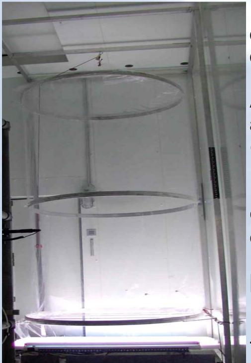
If made of glass, the walls of smog chambers are known to release Cl<sub>2</sub> from ozone and HCI by heterogeneous photochemistry. This artefact is avoided in our chamber, made of Teflon film (3500 I, FEP 200A, Dupont), (*Fig. 1*).
