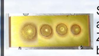
Samples of HULIS are deposited on a ZnSe-ATR-crystal by a home-made electrostatic precipitator and can be analysed using FTIR-spectroscopy.
