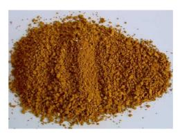
Figure 1: schwertmannite sorption materials produced at pilot scale in the EU-project ProMine
