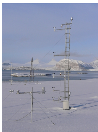
Figure 3: Flux-gradient measurement complex, 6 m tall meteorological gradient-tower and radiation measurement (MT2) of the Univ. of Bayreuth, monitoring area south-east of Ny-Ålesund (Svalbard), ARCTEX-2006 campaign.
