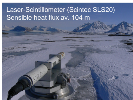
Figure 4: Laser Scintillometer, Scintec SLS20 (SLS) of the Univ. of Bayreuth, monitoring area south-east of Ny-Ålesund (Svalbard), ARCTEX-2006 campaign.
