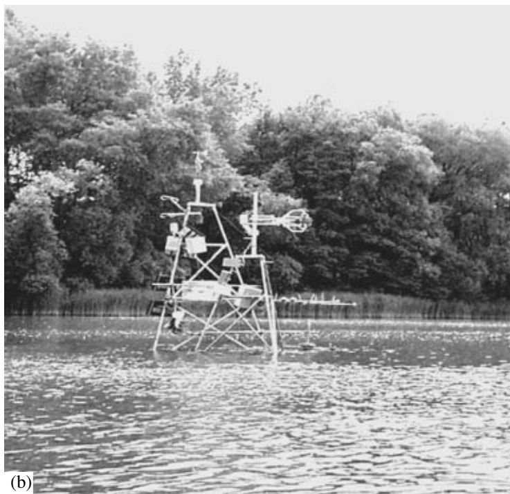
Fig. 5. (a) Great Kossenblatt Lake and (b) the tower for measurement of the vertical heat, moisture, and momentum fluxes together with radiation fluxes. The depth is 2.5 m.
