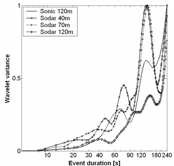
Figure 4: Normalised wavelet variance spectra of vertical wind fluctuations obtained by Sodar-Rass and sonic anemometer at July 29<sup>th</sup> 2003 15:45 – 16:10 CET during ECHO 2003.
