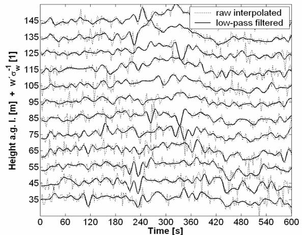
Figure 1: Time series of the normalised vertical wind speed of all observed levels at July 8<sup>th</sup> 2003 12:30 – 12:40 CET during WALDATEM-2003.
