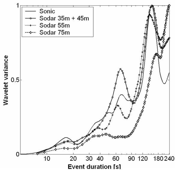
Figure 3: Normalised wavelet variance spectra of vertical wind fluctuations obtained by Sodar-Rass and sonic anemometer at July 8<sup>th</sup> 2003 12:30 – 12:55 CET during WALDATEM-2003.
