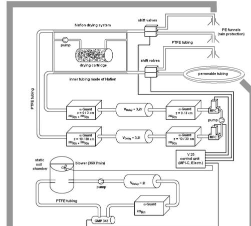
Figure 2: Radon measurement setup during EGER IOP2 (extended from Hens 2009).
