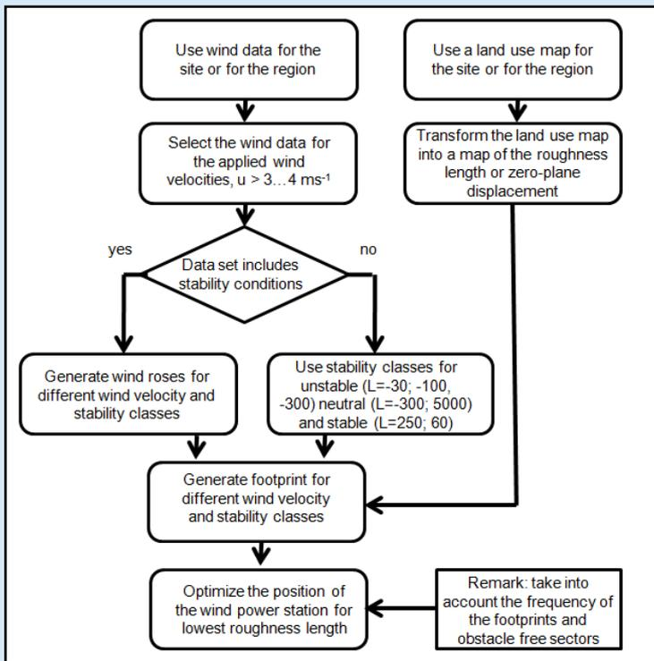
Fig. 3: Schema to find the best position for wind power stations based on wind roses, stability selections and footprint analysis. Finally the roughness length and zero-plane displacement height in the most frequent footprint sector must be minimized.
