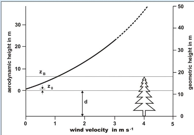
Fig. 1: Schematic wind profile above a canopy with the height  $z_B$ , the roughness length  $z_0$ , and the zero-plane displacement  $d$  and the definition of the aerodynamic height (left) in comparison to the geometric height (right), beginning at the physical ground (from [7], modified)
