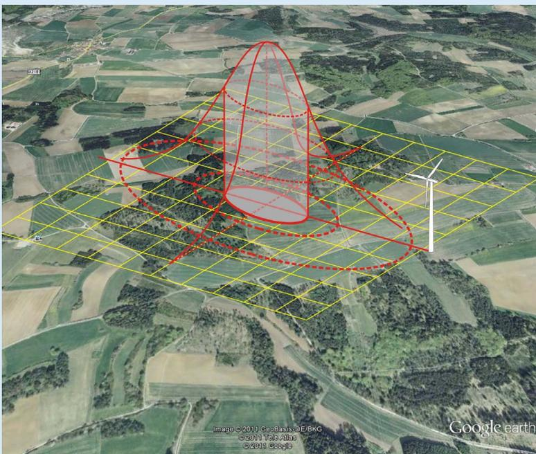
Fig. 4: Combination of a land use map, divided into different grid elements, and combined with the effect levels of the footprint model. The position of the wind power station is on the right (image from Google).
