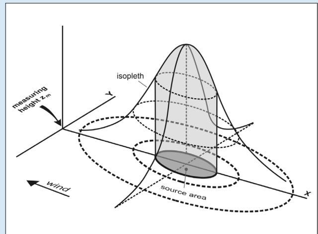
Fig. 2: Schematic view of the footprint function for a certain measuring height, with the strongest influence in the centre of the source area and lower influences in the outer parts characterized by effect levels (from [9], modified)
