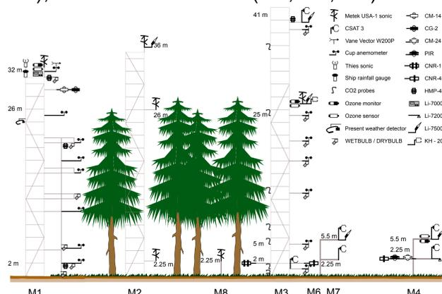
Figure 2: Installation of instruments during the measurements.
