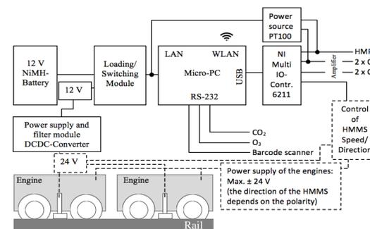
Figure 3: Schematic draft of the HMMS wiring. Sliding contacts tapped the power from the rails. The dashed lines show wiring of the engine power supply (24 V). Solid lines show wiring of the power supply of PC and sensors (12 V).
