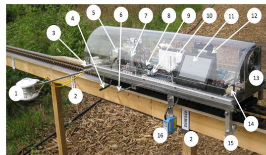
Figure 2: Lateral view on the HMMS. Find in Table 1 the specification of the numbers 1-12 and 16. The specification of the remaining numbers 13-15 are: 13: Fan for cooling the entire system 14: On board storage battery 15: Lateral holder to protect the HMMS for downfalls
