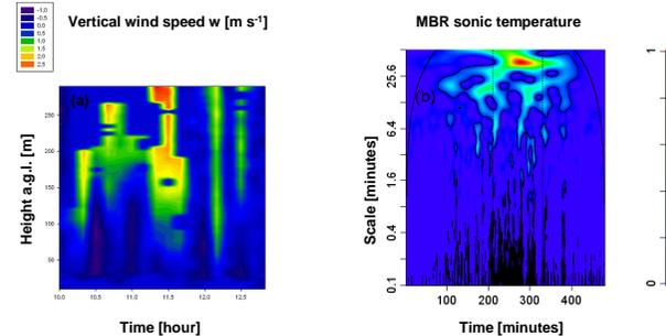
Figure 3: Vertical wind speed values  $w$  measured with the mini Sodar (a) on the clearing on 17 June 2008 during the FCE time (10:30-12:30) marked in Fig. 2. Figure 3b shows the wavelet power spectra of the MBR sonic temperature during the above-mentioned FCE time indicated by the black dashed vertical lines.
