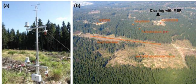
Figure 1: Modified Bowen ratio (MBR) mast (a) and location of the clearing in relation to the measuring setup (b).
