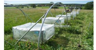
Fig. 3: <sup>13</sup>CO<sub>2</sub> pulse labelling chambers - cooled with thermal packs and fans - carbon tracer and acid reservoirs inside.
