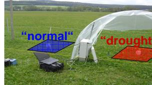
Fig. 2: Experiment setup: "Normal" and "drought"-plots alternating arranged in a row (5 repetitions each). Soil temp. and moisture have been logged on both.
