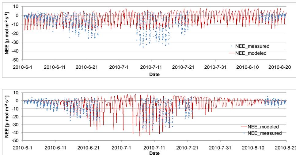
Figure 4. Daytime NEE measured and modeled by gap filling methods at KR-P. Above: traditional MMF; below: NMMF
