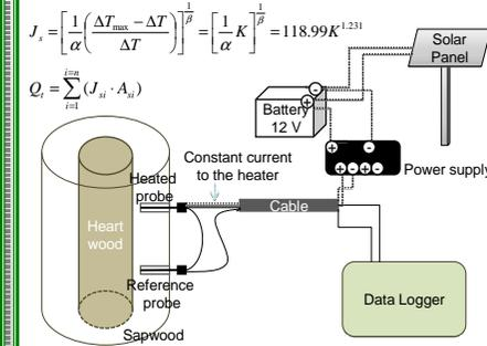
Fig. 4. Sapflow measurement, Thermal Dissipation Probe (TDP), introduced by Granier (1987)
