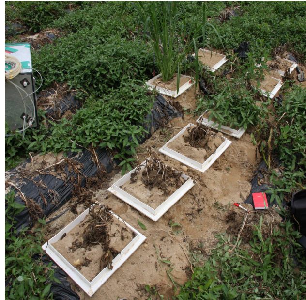
Figure 2: Installed soil frames (38 x 38 cm 2 ) as a base for the gas exchange chambers
