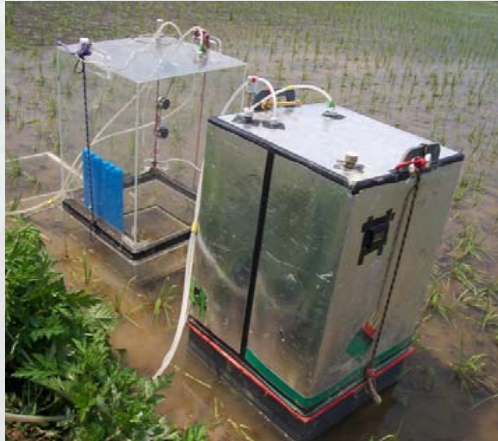
Figure 1: Applied light and dark gas exchange chambers for measuring the NEE and R_{eco}
