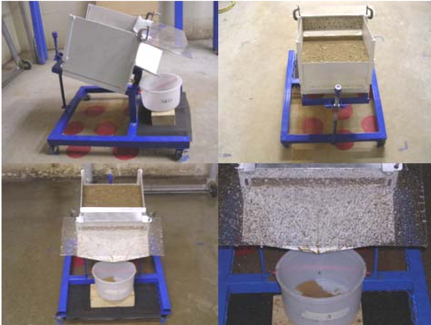
Tests for measuring runoff & sediment loss
