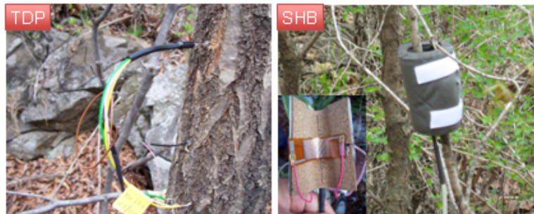
Fig3. (Left) Thermal Dissipation Probe (TDP) Method - Granier, 1987 (Right) Stem Heat Balance (SHB) Method - Sakuratani, 1981
