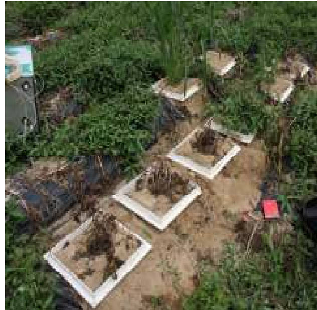
Figure 2: Installed soil frames ( 38 \times 38 \text{ cm}^2 ) as a base for the gas exchange chambers
