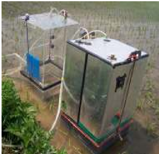
Figure 1: Applied light and dark gas exchange chambers for measuring the NEE and R_{eco}
