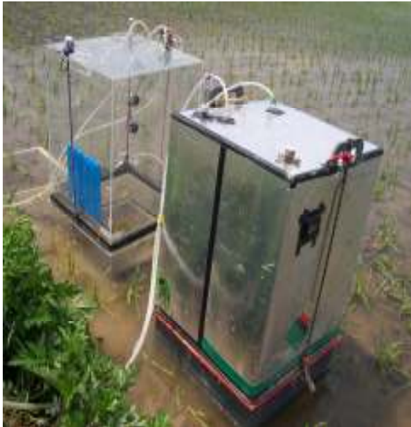
Figure 1: Applied light and dark gas exchange chambers for measuring the NEE and R_{eco}
