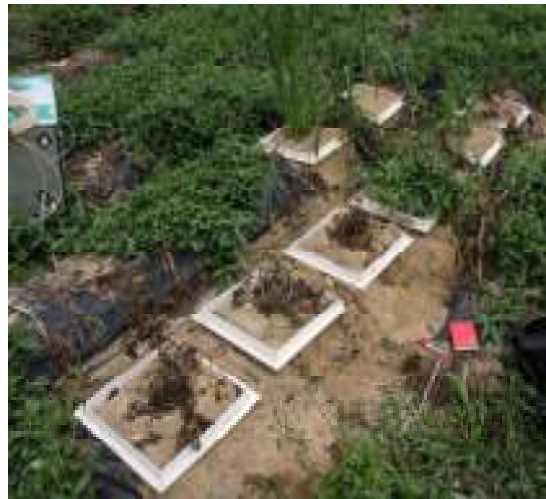
Figure 2: Installed soil frames (38 x 38 cm 2 ) as a base for the gas exchange chambers
