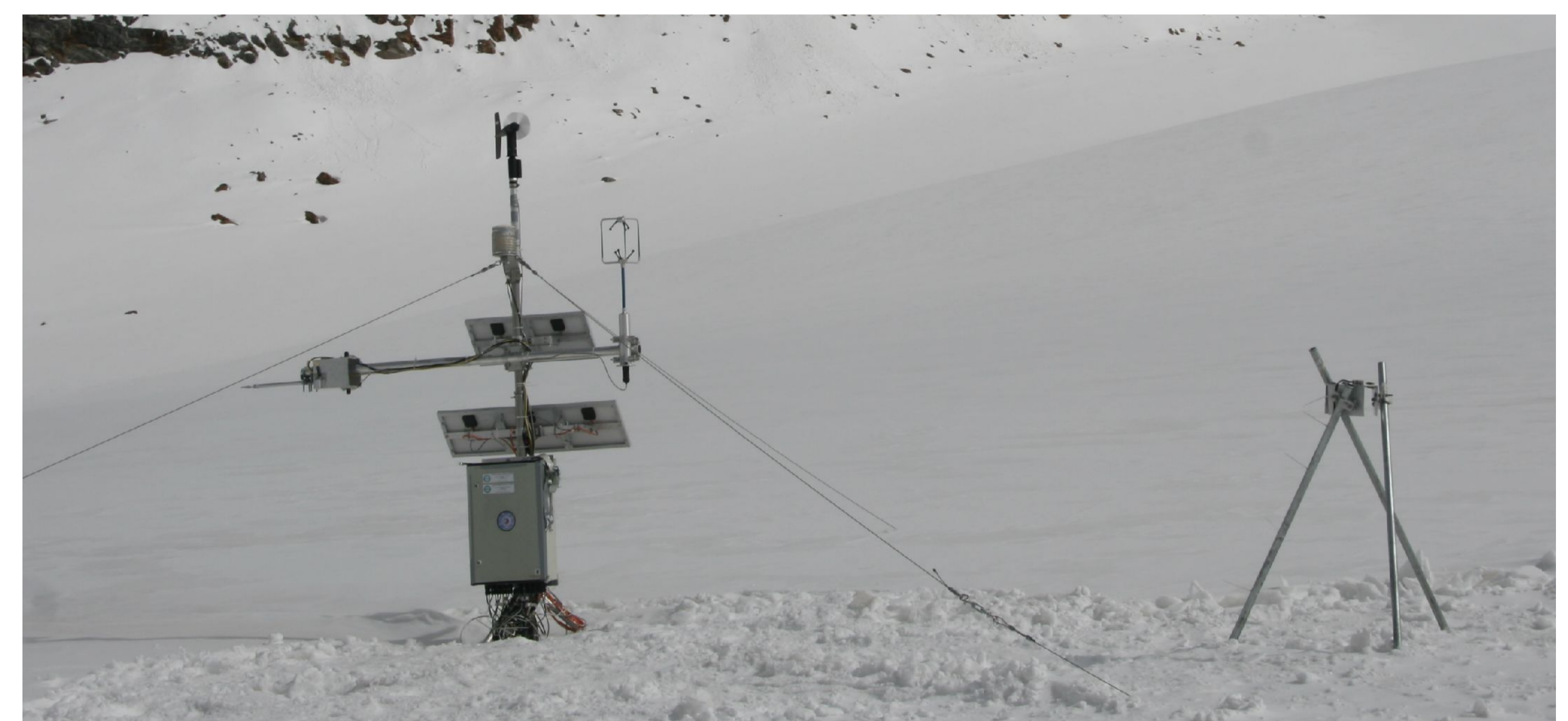
Fig 5: AWS 1 with Gill Windmaster and SR50 (right) in May 2010 on Zhadang Glacier
