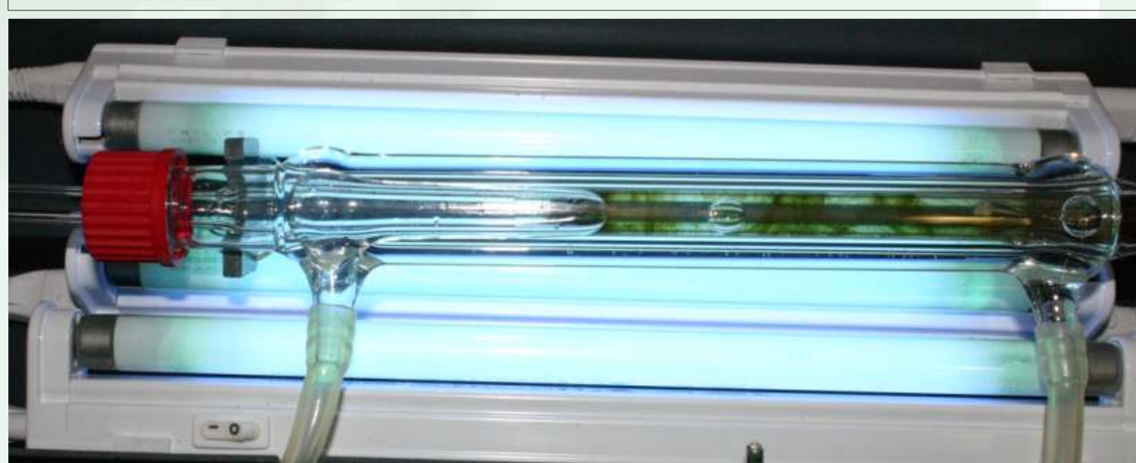
Heterogeneous flow-reactor illuminated by UV-lamps
