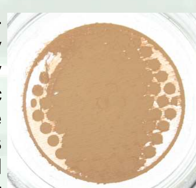
Glass fibre filter coated with SOA formed by the reaction of catechol with ozone and hydroxyl radicals at ultraviolet radiation.
