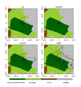
**Fig. 3.** Averaged cumulative footprint contours showing the footprint areas for 80 % (solid line) and 95 % (dotted line) of the total flux measured by eddy covariance for **(a)** all, **(b)** unstable, **(c)** neutral, and **(d)** stable conditions. x-axis and y-axis are distances from the mast (in m). The analysis was performed for all data from 29 August to 20 September 2005.
