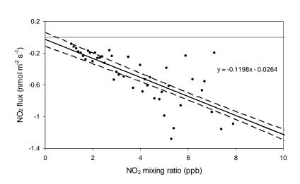
**Fig. 8.** Measured NO<sub>2</sub> flux as a function of the NO<sub>2</sub> mixing ratio (z = 2.0 m) from 29 August to 20 September 2005. Solid and dotted lines are the regression line and its 95% confidence interval, respectively. NO<sub>2</sub> fluxes were corrected for chemical reactions above the canopy and averaged for NO<sub>2</sub> mixing ratio bins of 0.1 ppb. Only data for  $G_r > 400$  Wm<sup>-2</sup> were included.
