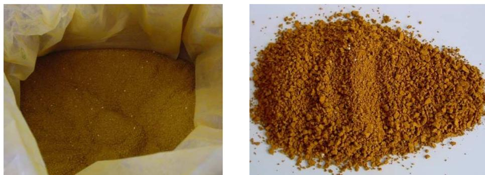
Figure 1: schwertmannite sorption materials produced at pilot scale in the EU-project ProMine
