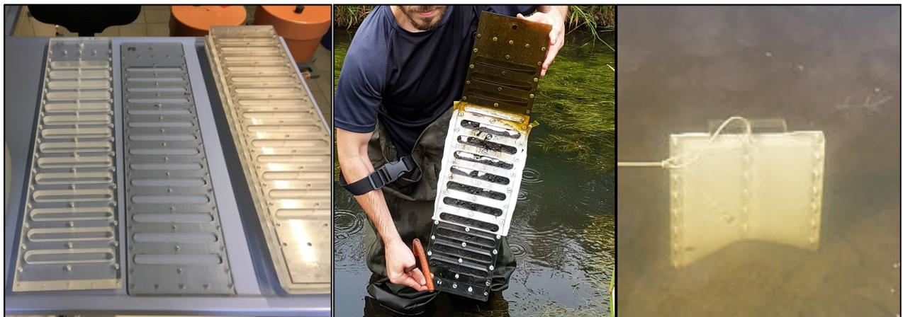
**Figure 1.** Left: Parts of the dialysis sampler (peeper). Middle: Image of the peeper after piercing the dialysis membrane. Right: Peeper installed in the riverbed.
