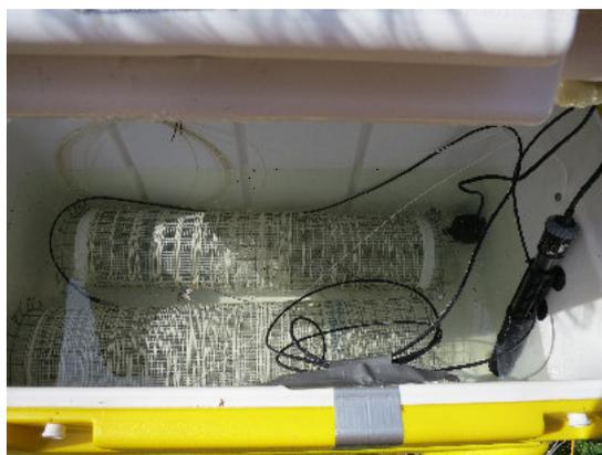
(II) Warmwaterbath with heater on the right side of the bath for 'span'-calibration
