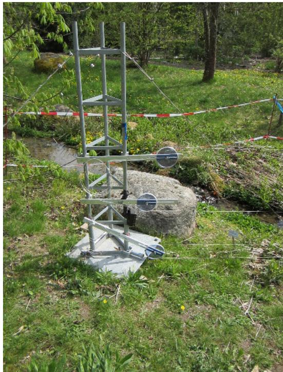
(I) Pulley-holder attached to the small tower at point A of the transect
