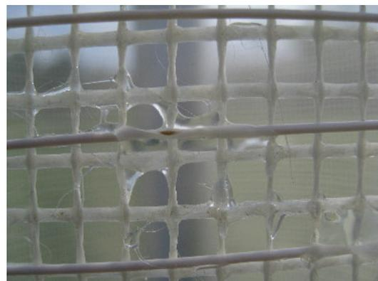
(IV) Melted PVC-coating at a glue dot
