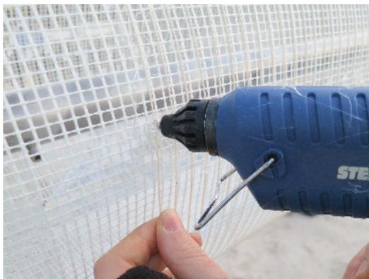
(III) Gluing fiber optic winding
