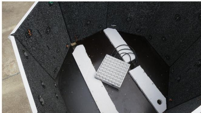
Figure 1.1: antennas of the Minisodar in the experiment set up
