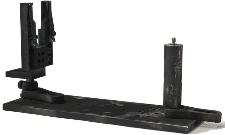
**Figure 4.5:** Close up of the construction for the photometric method: slide holder on the left, camera thread on the right, everything sprayed with a thermographic paint (emissivity of 0.97). The base plate ensures that the distance between sample and camera stays the same.
