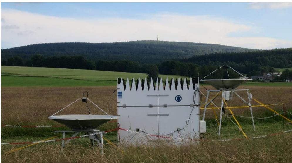
Figure 3: Metek Sodar RASS at Station 2
