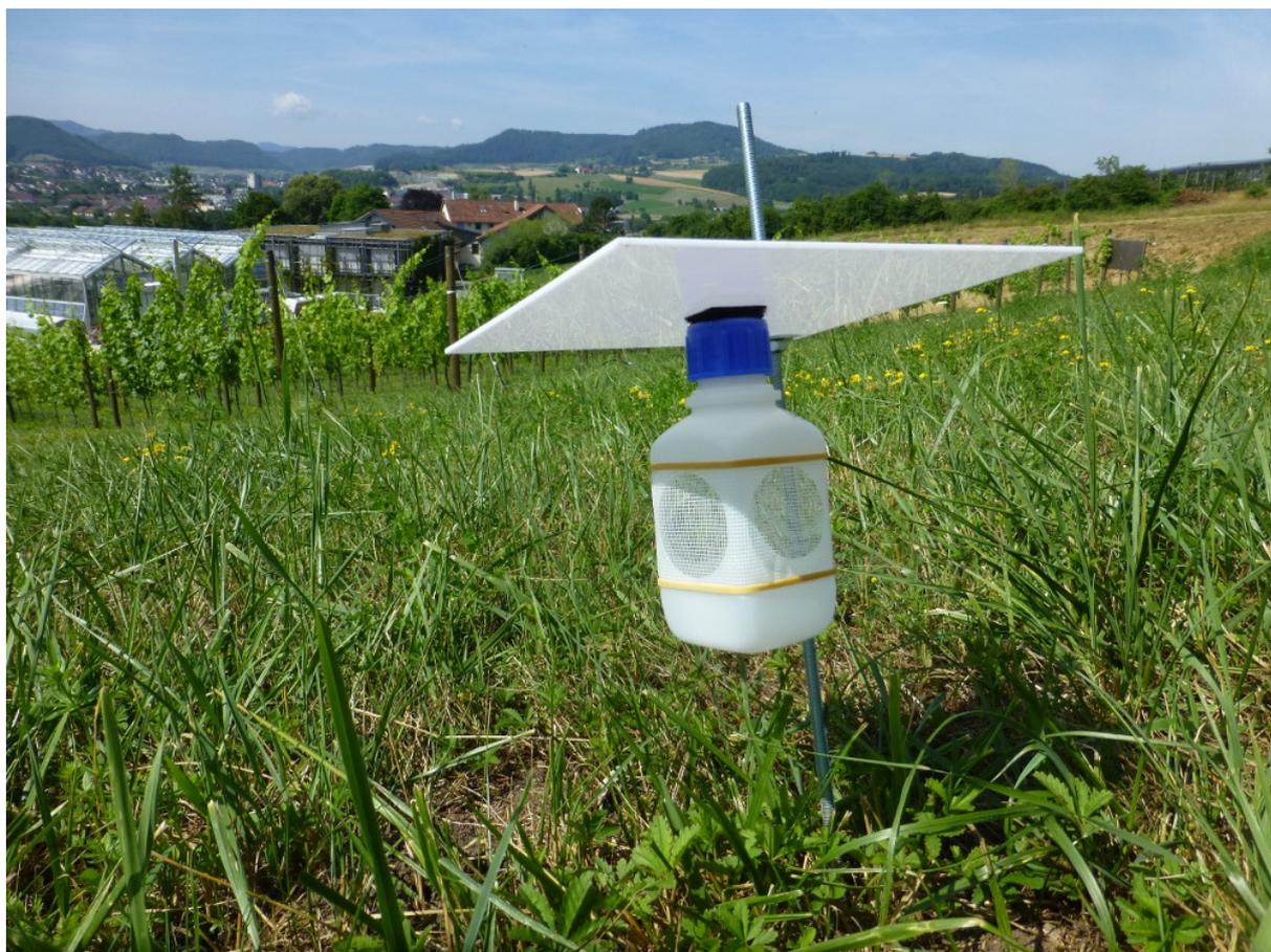
**Figure 3.9:** Acid trap passive sampler for cumulative air  $\text{NH}_3$  sampling.
