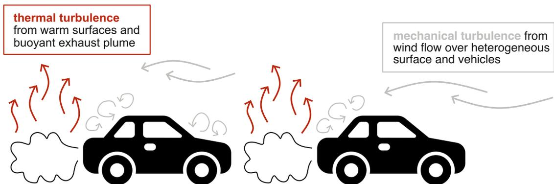
**Figure 4.:** Driving vehicles influence the turbulence regime in a street canyon both through mechanical and thermal mechanisms. This effect on the turbulence production is referred to as vehicle-induced turbulence (VIT)
