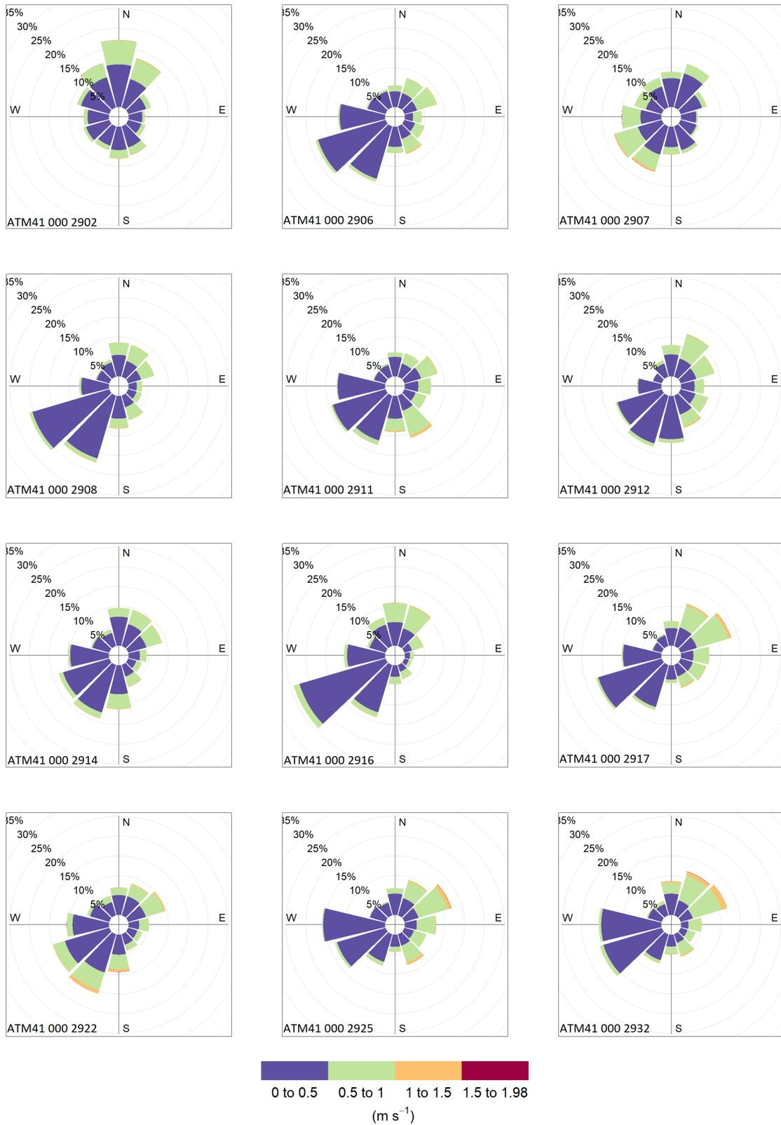
Figure B.6.: Comparison of the wind measurements of the micro weather stations; (data: 17 days with 5 min resolution  $\rightarrow N = 4837$ )
