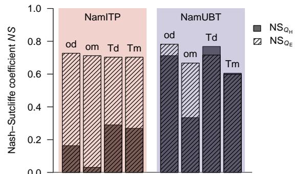
**Figure 5.** Nash-Sutcliffe coefficient ( $NS$ ) for turbulent fluxes (simulated vs. EBC-Bo corrected observations), left: NamITP, right: NamUBT. Grey bars denote  $NS$  for sensible heat flux and bars with shading lines denote  $NS$  for latent heat flux; individual blocks are coded as in Figure 4.
