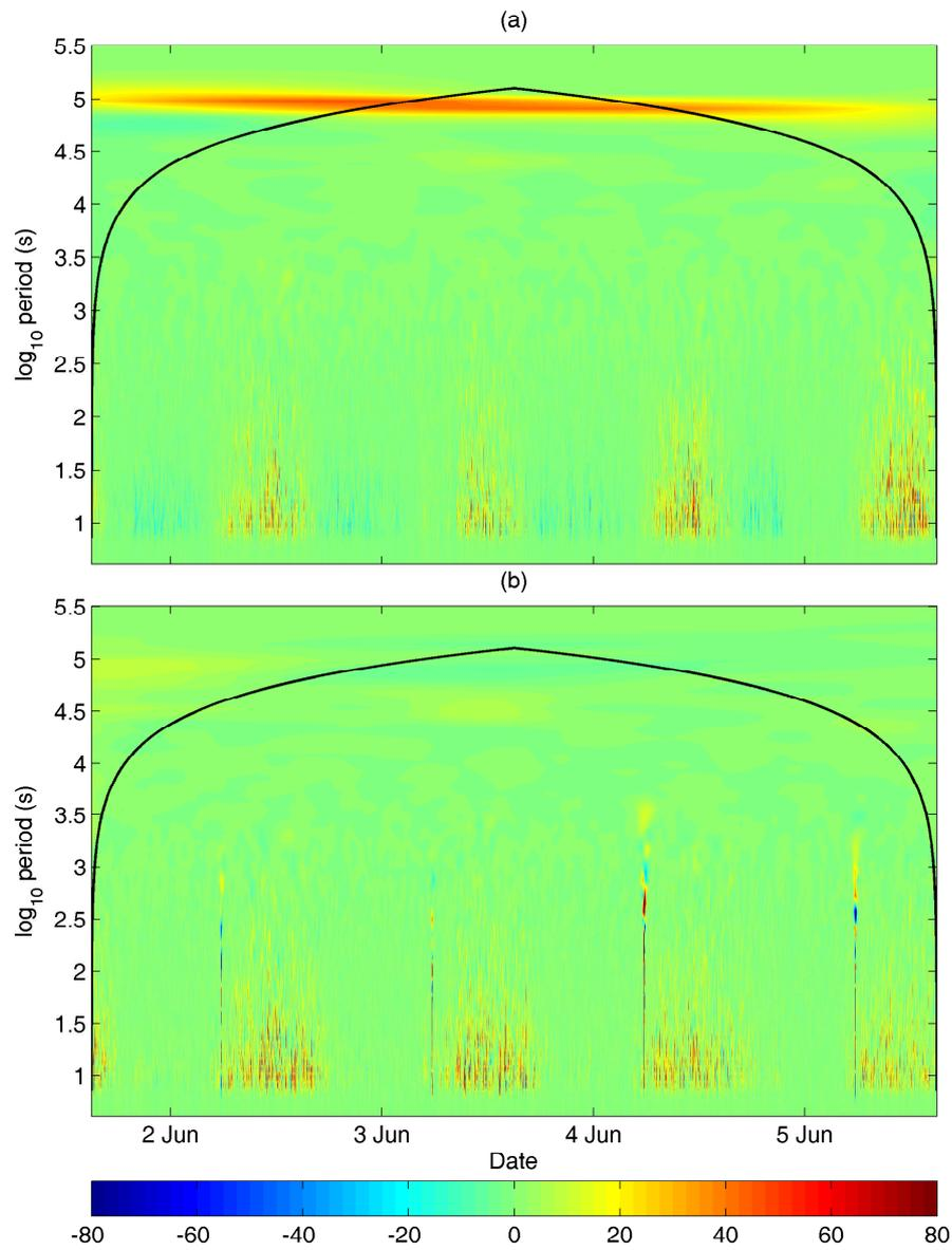
**Fig. 5** Wavelet cross-scalograms over the rye field during 1 June 2003, 1500 UTC - 5 June 2003, 1500 UTC of (a) sensible heat flux and (b) latent heat flux. The colour represents the value in  $\text{W m}^{-2}$ . The black solid line represents the cone of influence.
