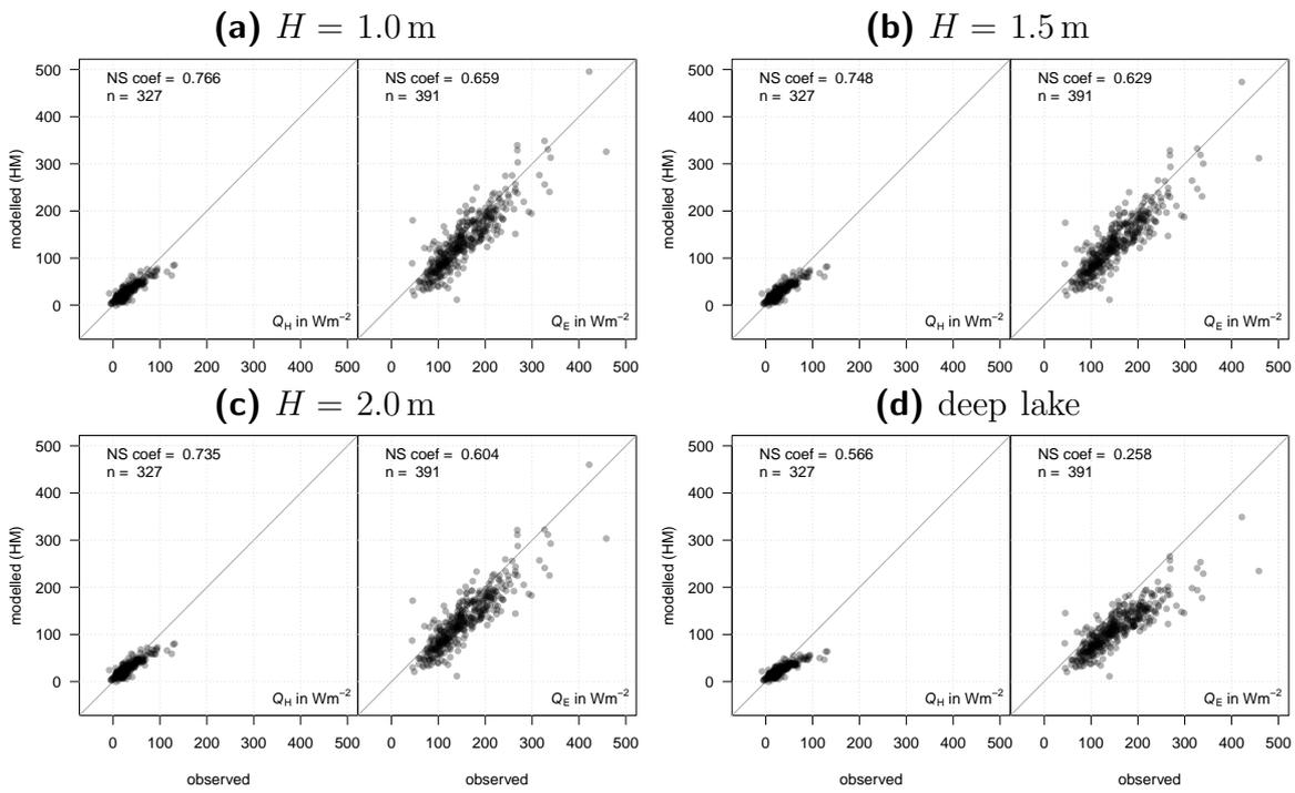
**Figure 4.4.** Turbulent flux observations above the shallow lake versus HM model simulations for different assumptions of lake depth  $H$  within the eddy-covariance footprint; flux simulations in panel **d** are computed without shallow water extension.
