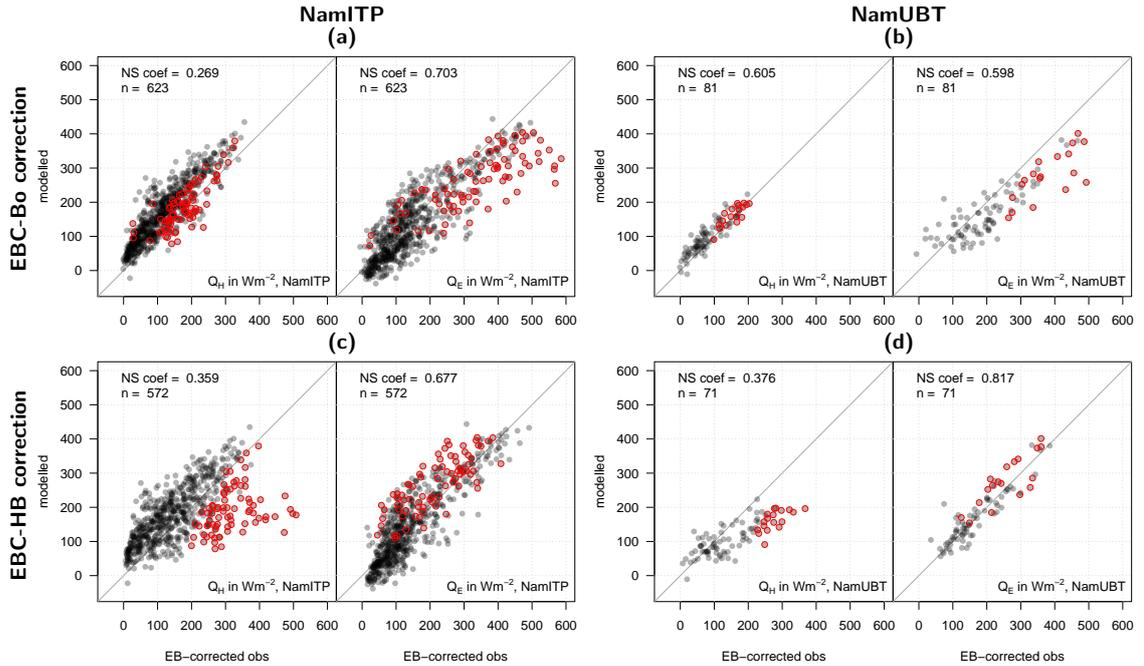
**Figure 11.** Turbulent flux observations versus model simulations, **measured** parameters, TP version, at NamITP (a,c) and NamUBT (b,d); Observations are displayed using the EBC-Bo correction (a,b) and the EBC-HB correction (c,d). The red points indicate data with  $-Res > 150 \text{ W m}^{-2}$  (not included in the analysis).
