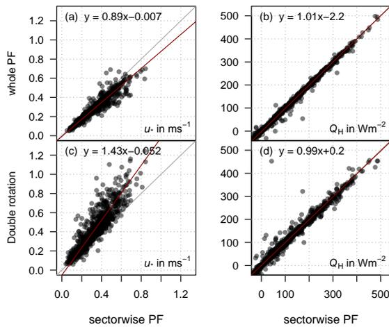
**Fig. 5.** Comparison of the sector-wise planar-fit rotation vs. planar-fit rotation for all wind directions (a, b) and vs. double rotation (c, d) for the friction velocity (a, c) and the sensible heat flux (b, d); data set A, DAT 600, was used, only from the undisturbed sector and with high quality (flag 1–3 according to Foken et al., 2004).
