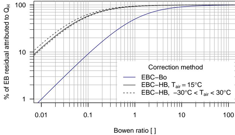
**Figure 3.3.** General effect of the energy balance correction methods according to the Bowen ratio (EBC-Bo) and according to the buoyancy flux (EBC-HB); the percentage of the residual attributed to  $Q_H$  is shown in dependence on  $Bo$ ; EBC-HB weakly depends on air temperature  $T_{\text{air}}$  and the dashed lines indicate the range of the relationship at  $-30^\circ\text{C} < T_{\text{air}} < 30^\circ\text{C}$ ; modified from Charuchittipan et al. (2013, Appendix E)
