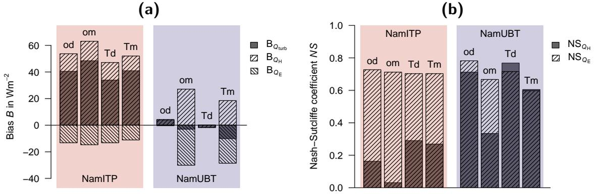
**Figure 4.2.** Bias (a) and Nash-Sutcliffe coefficient  $NS$  (b) of turbulent fluxes (simulated vs. EBC-Bo corrected observations), NamITP corresponds to grass<sup>-</sup>, NamUBT to grass<sup>+</sup>; the individual blocks show **od**: original SEWAB version, default parameters; **om**: original SEWAB version, measured parameters; **Td**: TP version, default parameters; **Tm**: TP version, measured parameters. Modified from Babel et al. (2013, Appendix C)
