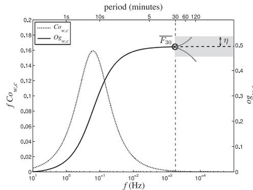
**Fig. 1** The short term average time series can estimate the turbulent flux at a 30 minute period ( $\overline{F_{30}}$ ) and its evolution after that (gray solid lines in a gray band). The error band of width  $2\eta$  (gray band) was defined for identifying the ogive case. See Table 2 for ogive case definition.
