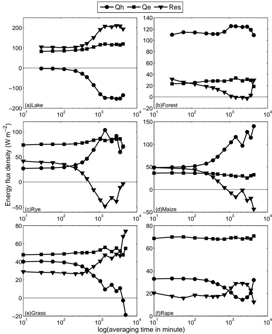
**Fig. 4** Block ensemble averages of sensible heat flux and latent heat flux (Eq. 17 with  $c$  is temperature and absolute humidity), and their corresponding residuals, during 1 June 2003, 1500 UTC - 5 June 2003, 1500 UTC of selected sites in the LITFASS-2003 experiment: (a) lake, (b) forest, (c) rye, (d) maize, (e) grass and (f) barley.
