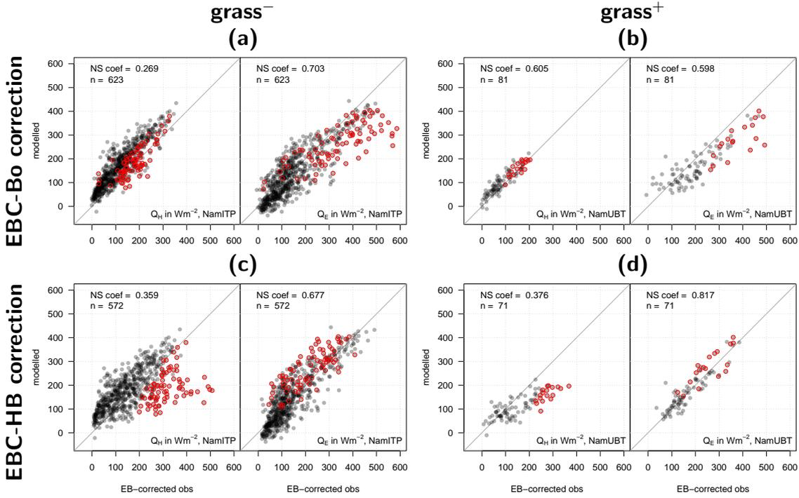
**Figure 4.3.** Turbulent flux observations versus model simulations, **measured** parameters, TP version, for grass<sup>-</sup> (a, c) and grass<sup>+</sup> (b, d); Observations are displayed using the EBC-Bo correction (a, b) and the EBC-HB correction (c, d). The red points indicate data with  $-Res > 150 \text{ W m}^{-2}$  (not included in the analysis). From Babel et al. (2013, Appendix C).
