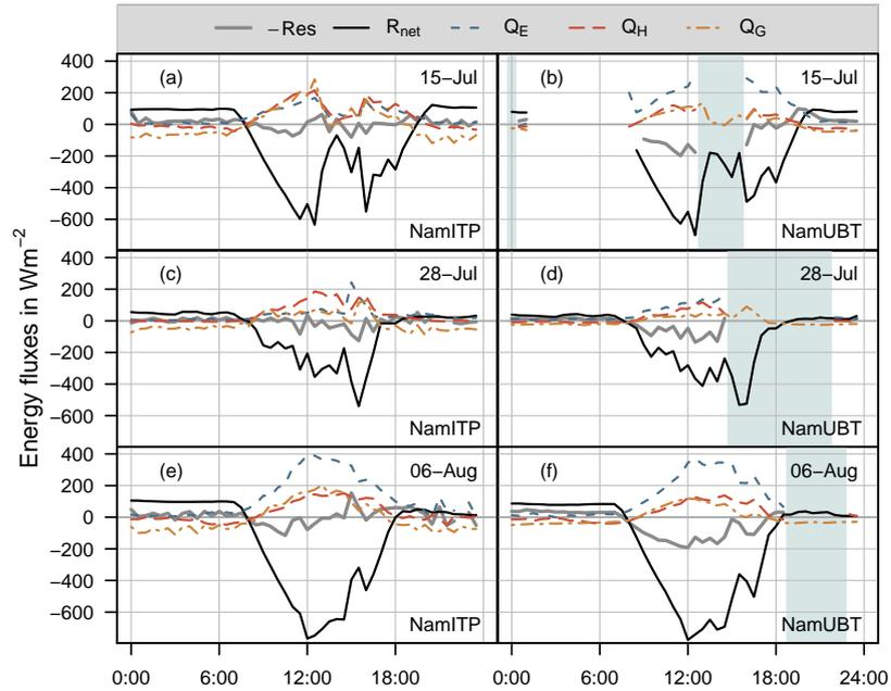
**Figure 2.** Diurnal cycles of the observed energy fluxes at Nam Co and the balance residual  $Res$  on 15 July (a,b), 28 July (c,d) and 6 August, 2009 (e,f) at NamITP (a,c,e) and NamUBT (b,d,f); blue shaded areas for NamUBT indicate missing data due to insufficient fetch (wind direction from the lake).
