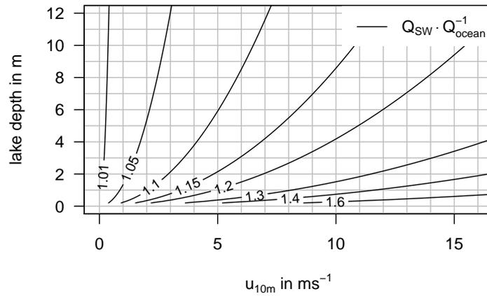
**Figure 3.4.** Sensitivity of the shallow water term on lake depth  $H$  and wind velocity in 10 m height  $u_{10m}$ : Isolines show the relative increase of deep water fluxes  $Q_{SW} \cdot Q_{ocean}^{-1}$  depending on  $u_{10m}$  and  $H$
