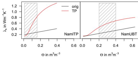
**Figure 8.** Simulated thermal conductivity  $\lambda_s$  in dependence on soil moisture  $\Theta$ ; grey rectangles indicate the observed range of upper soil moisture for the respective station.
