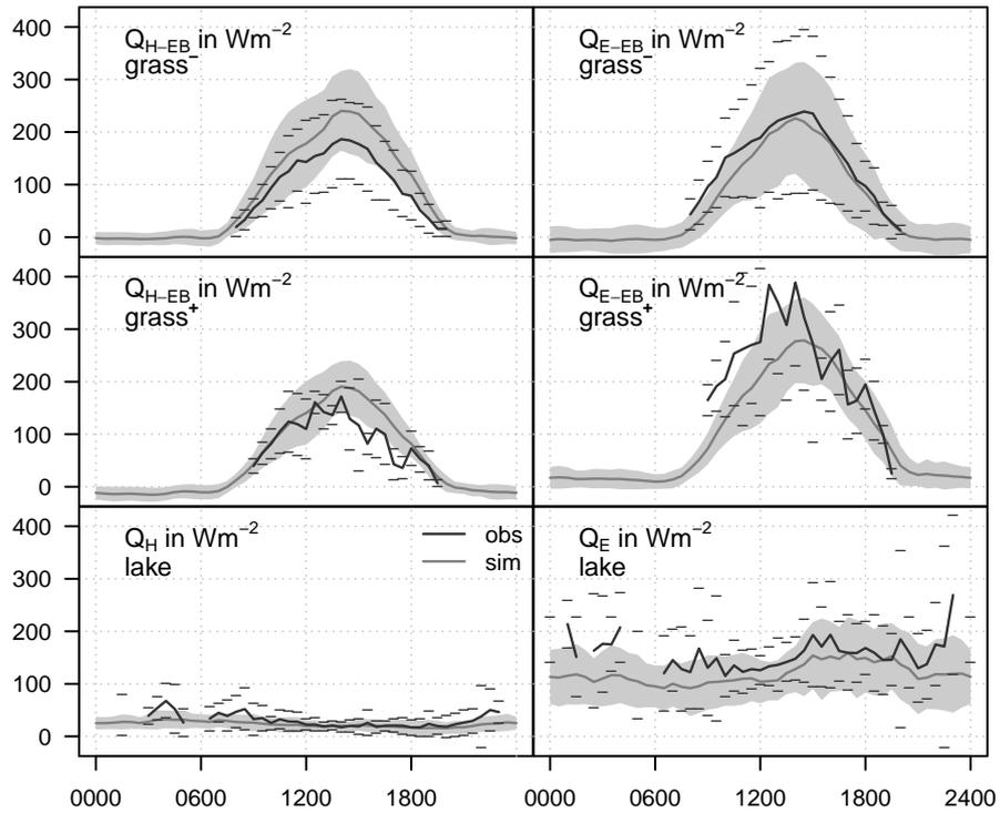
**Figure 4.6.** Diurnal cycle of observations and simulations at Nam Co 2009. Land surface observations have been corrected according to the Bowen ratio (EBC-Bo), respective simulations have been run in the TP version using the measured parameters. Solid lines represent mean fluxes while horizontal bars and grey shaded areas denote respective standard deviations for observations and simulations. From Biermann et al. (2013, Appendix D).
