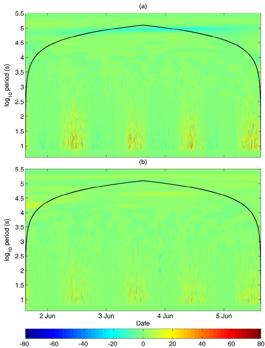
**Fig. 6** Wavelet cross-scalograms over the grassland during 1 June 2003, 1500 UTC - 5 June 2003, 1500 UTC of (a) sensible heat flux and (b) latent heat flux. The colour represents the value in  $\text{W m}^{-2}$ . The black solid line represents the cone of influence.
