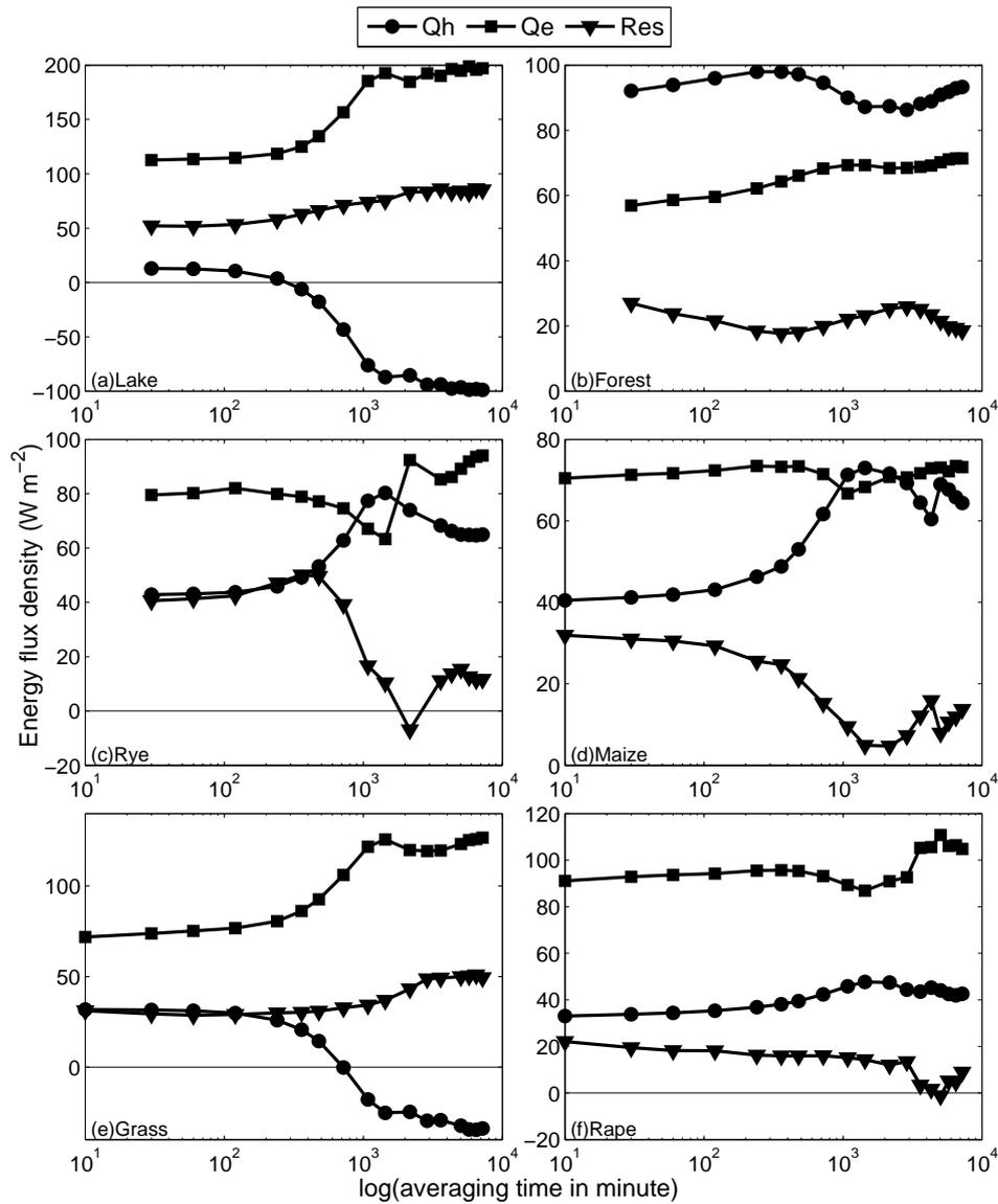
**Fig. 2** Block ensemble averages of sensible heat flux and latent heat flux (Eq. 17 with  $c$  is temperature and absolute humidity), and their corresponding residuals, during 2 June 2003, 1800 UTC - 18 June 2003, 0000 UTC of selected sites in the LITFASS-2003 experiment: (a) lake, (b) forest, (c) rye, (d) maize (reproduction of Mauder and Foken (2006)), (e) grass and (f) barley.
