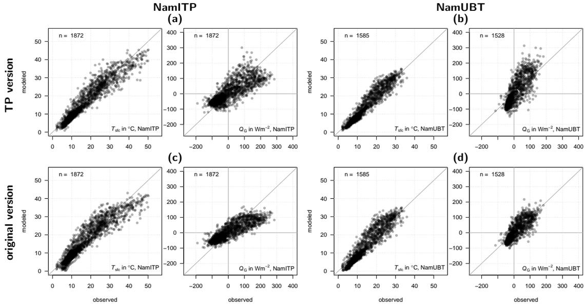
**Figure 6.** Observations of surface temperature and ground heat flux versus model simulations, **measured** parameters at NamITP (a,c) and NamUBT (b,d); simulations are displayed for TP version (a,b) and original version (c,d).
