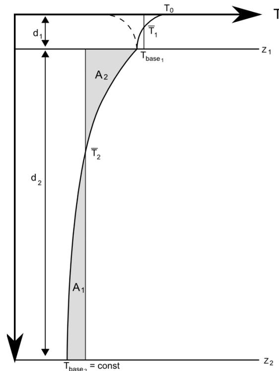
Fig. 4. Conceptual drawing of the assumed quadratic subgrid soil temperature profile and the associated parameters. In order to derive  $\bar{T}_1$  and  $\bar{T}_2$  geometrically the areas  $A_1$  and  $A_2$  must be equal.
