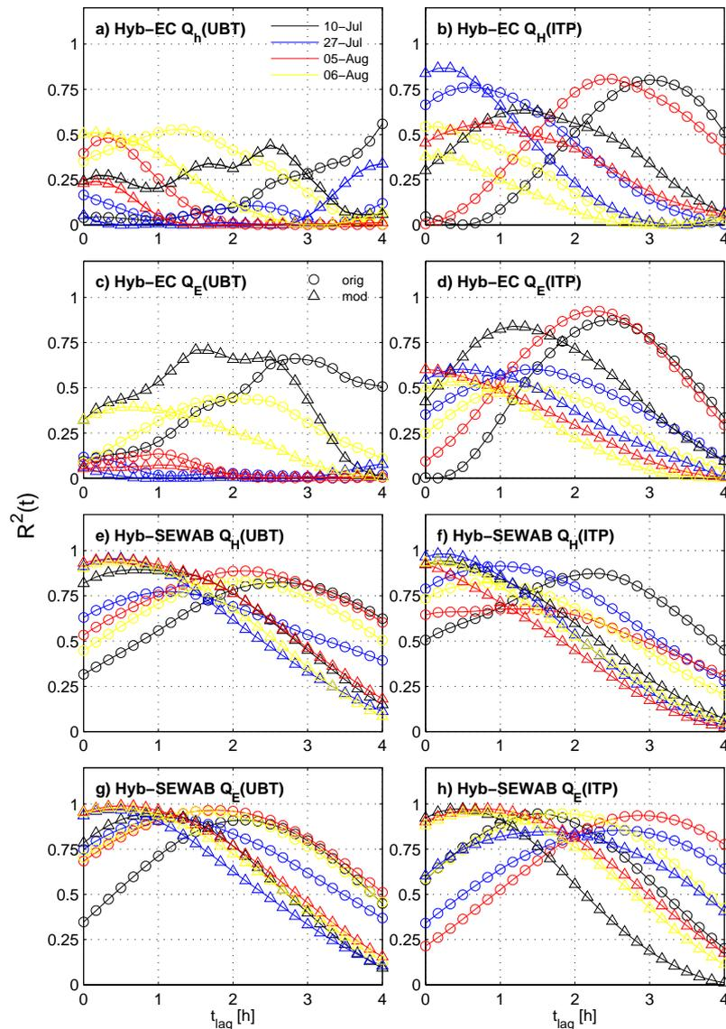
**Fig. 8.** Cross correlation  $R^2(t)$  of simulated fluxes against flux reference shifted by  $t_{\text{lag}}$  as multiples of 10 minutes for each of the four days simulated with the original and modified Hybrid. The maximum number of elements used in the calculation of  $R^2$  for each curve can be taken from Table 3.
