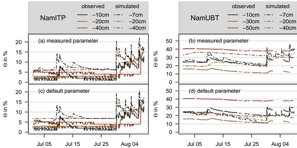
**Figure 7.** Timeseries of observed and simulated volumetric soil moisture content at various depths, **TP version**, at NamITP (a,c) and NamUBT (b,d); simulations are displayed for measured parameters (a,b) and default parameters (c,d). Note, that simulated soil depths do not match the observed soil depths in case of NamUBT.
