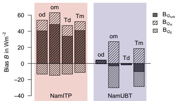
**Figure 4.** Bias of turbulent fluxes (simulated vs. EBC-Bo corrected observations), left: NamITP, right: NamUBT. Bars with ascending shading lines denote sensible heat flux bias, descending shading lines latent heat flux bias and the sum is the turbulent heat flux bias (grey bars); the individual blocks show **od**: original SEWAB version, default parameters; **om**: original SEWAB version, measured parameters; **Td**: TP version, default parameters; **Tm**: TP version, measured parameters.
