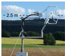
Fig.1: EC station (LI-COR LI-7500 & Campbell CSAT3)
