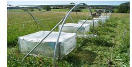
Fig.7:  $^{13}\text{C}_2$  pulse labeling chambers - cooled with thermal packs and fans
