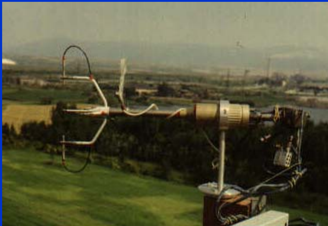
The Russian phase-shift sonic anemometer (more recent type, 1986)
