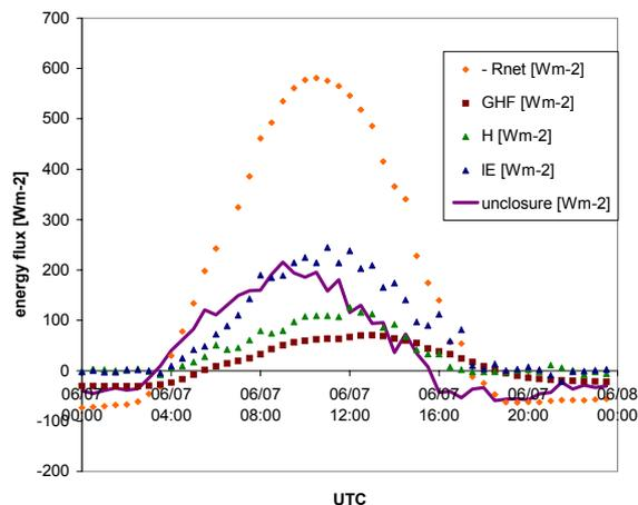
Figure 4: Results of energy flux measurements **without** the application of the presented approaches of **quality assurance and soil heat storage**. Micrometeorological site LITFASS-2003 A6, corn field in Brandenburg/Germany. June 7<sup>th</sup> 2003.
