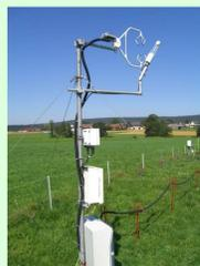
Fig. 2: Turbulence measurement complex (with LI-7500 IRGA and CSAT3 ultra sonic)
