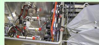
Fig. 8: REA system with 90cm foil balloons and the sampling unit with drying traps
