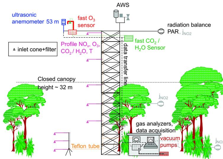
**Fig. 3.** Scheme of the cumulative experimental setup of the tower site at the Reserva Biológica Jarú (RBJ) during LBA-EUSTACH 1 and 2 campaigns. Measurements performed periodically are displayed in light gray (e.g.  $\text{NO}_2$  photolysis rate  $j_{\text{NO}_2}$  was measured alternately at three heights).
