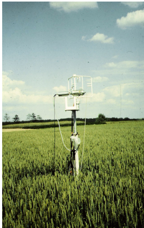
Fig 3: Sonic anemometer and Lyman-alpha-hygrometer of the Meteorological Main Observatory Potsdam during intercomparison measurements at Müncheberg (photo: Th. Foken).
