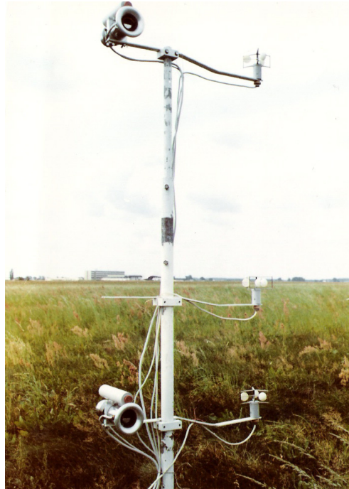
Fig. 4: Mast for the parameterization of turbulent fluxes of the Meteorological Main Observatory at Potsdam, consisting of anemometers at three and psychrometers at two heights, during measurements at the Berlin-Schönefeld Airport in 1985 (photo: Th. Foken).
