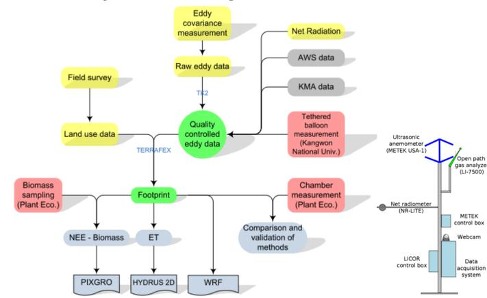
Figure 3: Method of the research (right: installation of the instruments)
