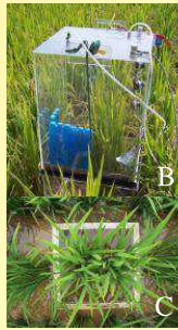
Figure 1: A) Experimental set up for the CO 2 chamber measurements in the crop fields. B) Installed light chamber during the CO 2 exchange measurements in the rice field. C) Top down detail picture of a rice plot.
