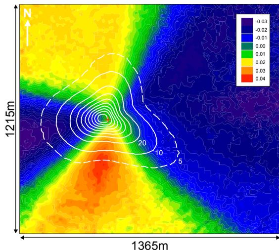
Figure 5: Mean value of the vertical wind component  $w$  [m/s] after performing the Planar Fit rotation method (Wilczac et al., 2001). The footprint climatology for all stratification cases is indicated by the white isolines, with the tower position marked by the red cross.
