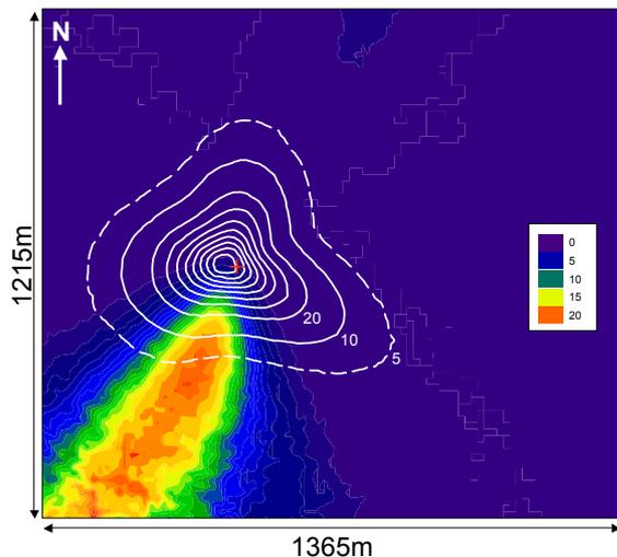
Figure 4: Spatial distribution of the quality assessment results for the vertical wind component. The footprint climatology for all stratification cases is indicated by the white isolines, with the tower position marked by the red cross. Colours indicate the percentage of unrotated mean vertical wind speeds exceeding the threshold of  $0.35 \text{ m s}^{-1}$ .
