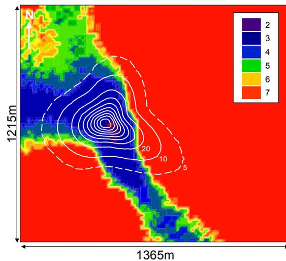
Figure 3: Spatial distribution of the quality assessment results for the sensible heat flux. The footprint climatology for all stratification cases is indicated by the white isolines, with the tower position marked by the red cross. Colours indicate the average data quality for each matrix cell, ranging from 1 (best) to 9 (worst).
